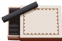
litho crayon Rectangular stick of grease chalk used to draw a figure on a lithographic stone.
