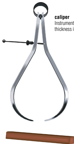
red ocher pencil Stick of hematite (iron oxide) used to produce a sketch on paper; the sketch is then transferred to the stone.
