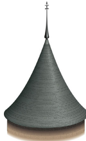
conical broach roof Conical roof usually surmounting a turret.
