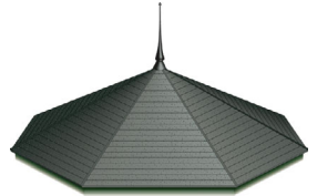
rotunda roof Roof with several triangular sides on a polygonal base.
