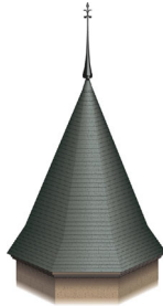
sloped turret Many-sided roof whose slope is steep at the summit and gentle at the base.
