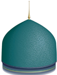
bell roof Roof covering the hollow semicircular vault of a building (dome).
