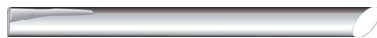
pumice correcting pencil Instrument used to polish the stone and make corrections to the figure.
