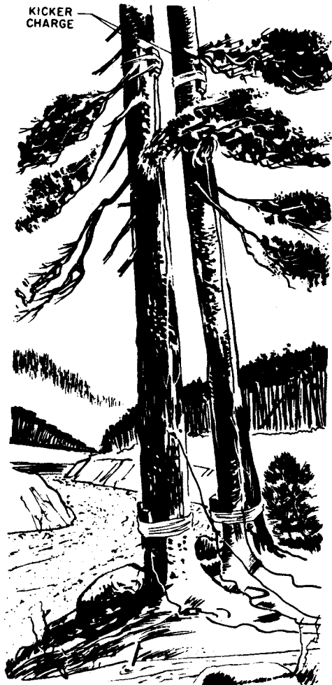
Figure 5 External and Kicker Charge Placement
