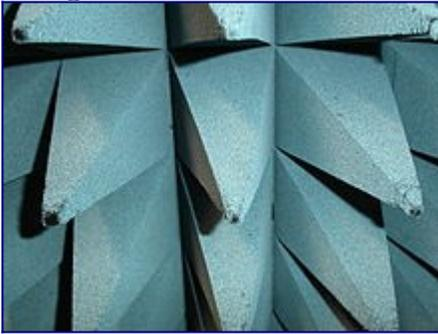
Pyramid RAM. The grey paint helps to protect the delicate radiation-absorbent material.
