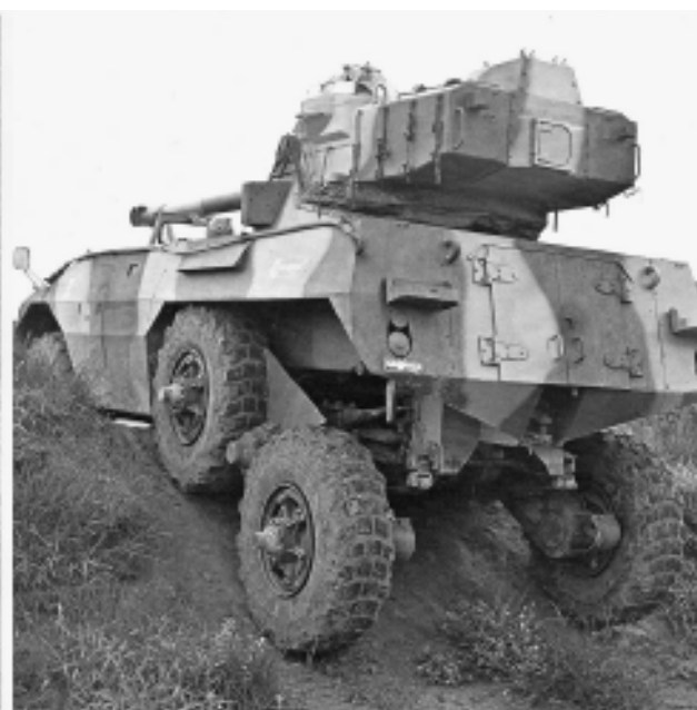
The Sucuri tank destroyer in promotional material (left) and its Engesa “boomerang” suspension in use (right)
