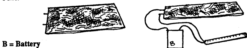
Pressure mats and circuit connection
