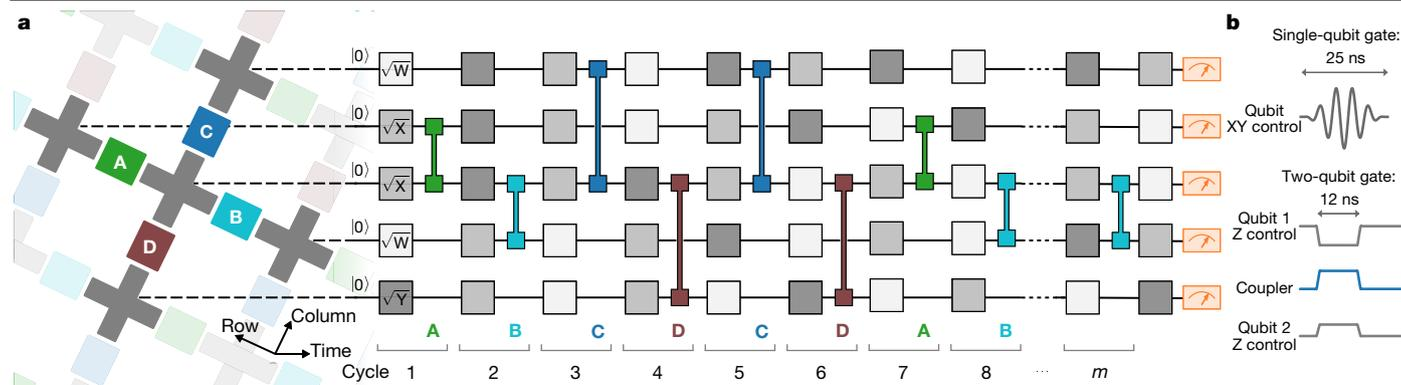
**Fig. 3 | Control operations for the quantum supremacy circuits. a**, Example quantum circuit instance used in our experiment. Every cycle includes a layer each of single- and two-qubit gates. The single-qubit gates are chosen randomly from  $\{\sqrt{X}, \sqrt{Y}, \sqrt{W}\}$ , where  $W = (X + Y)/\sqrt{2}$  and gates do not repeat sequentially. The sequence of two-qubit gates is chosen according to a tiling pattern, coupling each qubit sequentially to its four nearest-neighbour qubits. The
