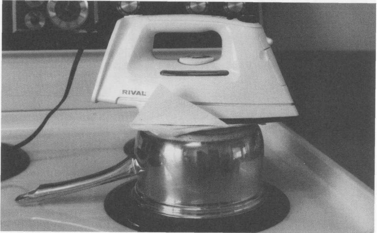
A clothes iron, an upside-down saucepan, and napkin make a very effective laminator for the poor man.
